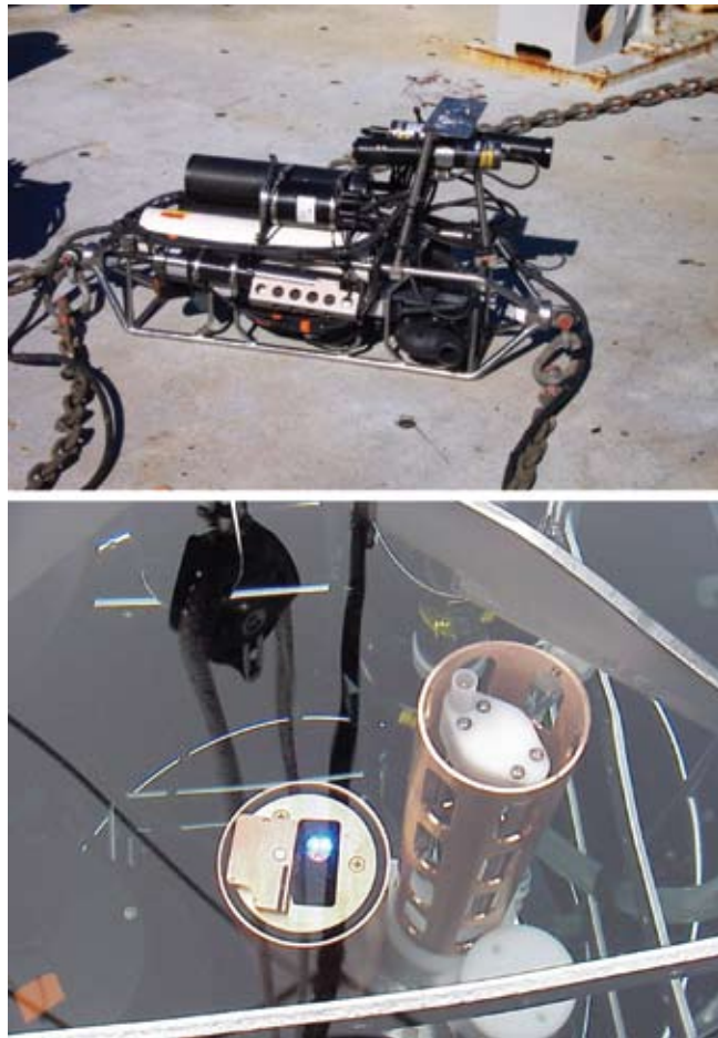
Figure 3. (Top) Optical package used for measuring several inherent and apparent optical properties during the MOSEAN field trials. (Bottom) The WET Labs water quality monitoring (WQM) optical measurement system equipped with special anti-biofouling devices.
