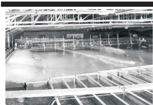
Figure 1. The LSTF during a plunging-wave case, showing the flow channels (bottom) and the instrument bridge (top) carrying the various instruments. The locations of the FOBS sensors (vertical) are indicated by referring the
